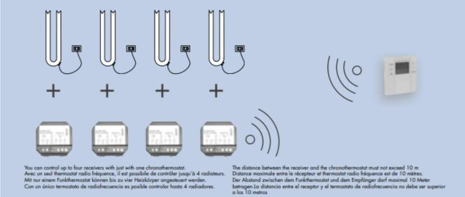
You can control up more radiators, for a maximum power of 2000 watt, with just one receiver
