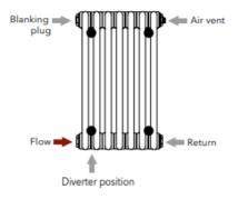
The flow must be connected on the side closest to the flow diverter
