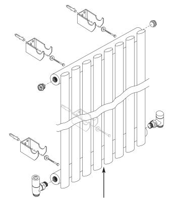
Only connect the header with the 'flow diverter' to the system. Visually or physically check this before proceeding (you will not be able to see all the way through the correct header, it is blanked off at its mid point) The top header is clear of any obstruction.
